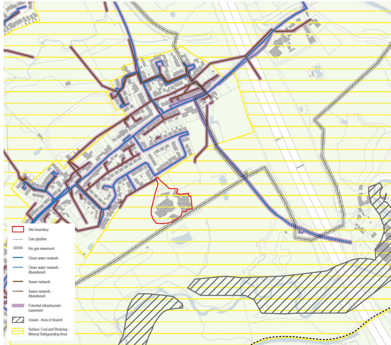
Figure 8: Existing sewage and water infrastructure
